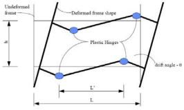
Figure 7-1 - Desired Plastic Frame Behavior
