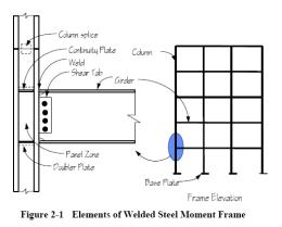
foregoing The is the same detail incorporated in the ASEP Guide "Earthquake Resistant Design of Structures 1991 Ed" unfortunately; this guide has not been replaced nor superseded to reflect the current State of knowledge regarding the problems associated with this connection detail in the light of the Northridge Earthquake experience.
